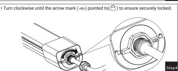
To ensure waterproof protection of luminaire, the cable gland should be tighten properly with minimum torque of 1.2Nm.
